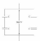
$C_{eq} = \frac{C}{2} + \frac{C}{2} = C$ . So the total capacitance is the same as each individual capacitor, and the voltage is spilt over each so that V = 480 V. Another solution is two capacitors in parallel that are in series with two others in parallel.
